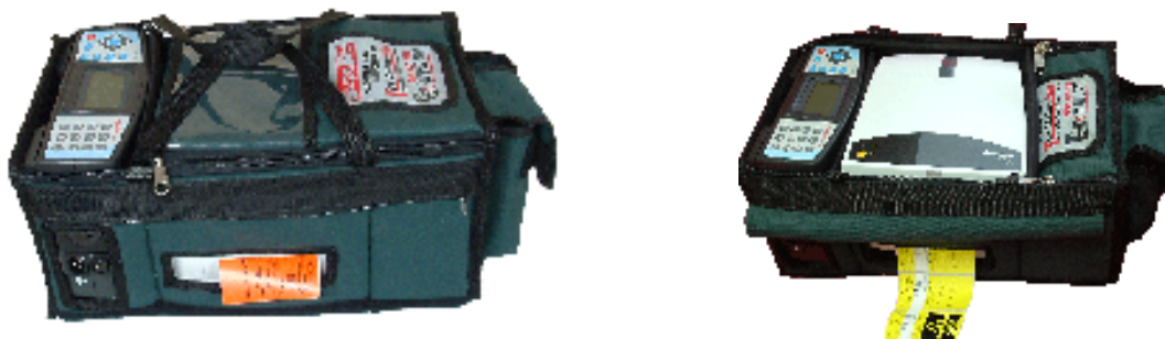
Fig. 7.4. Example of a complete system for printing appliance labels (AlphaPAT + Intermec C4 printer)
