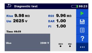
Figure 7.13: Examples of Diagnostic test result
