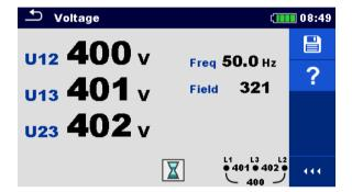
Figure 7.5: Examples of Voltage measurement in three-phase system
