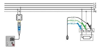
Figure 7.29: Connection of Plug commander and 3-wire test lead
