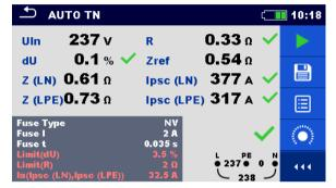
Figure 8.11: Examples of AUTO TN measurement results
