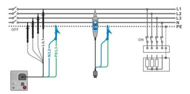
Figure 7.11: Connection of 3-wire test lead and Tip commander (U<sub>N</sub>≤1 kV)
