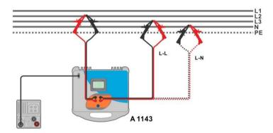
Figure 7.42: Phase-neutral or phase-phase high precision Line impedance measurement – Connection of A 1143
