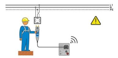
Figure 1.1: Reversed L and PE conductors (plug commander)
