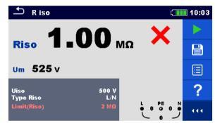
Figure 7.9: Examples of Insulation resistance measurement result
