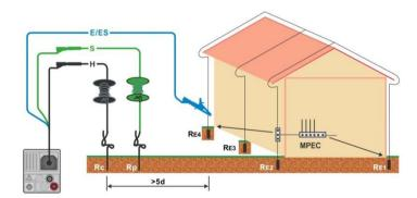
Figure 7.50: Resistance to earth, measurement of a lighting protection system
