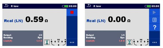
Figure 7.21: Result with old and new calibration values
