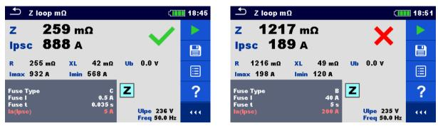
Figure 7.37: Examples of high precision Loop impedance measurement result
