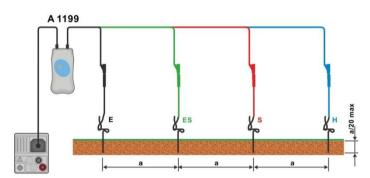
Figure 7.56: Specific earth resistance measurement
