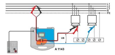
Figure 7.36: Contact voltage measurement – Connection of A 1143
