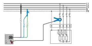
Figure 7.62: Harmonics measurement
