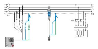
Figure 7.7: Connection of 3-wire test lead and Tip commander (U<sub>N</sub>≤1 kV)
