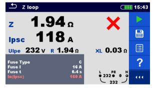
Figure 7.30: Examples of Loop impedance measurement result
