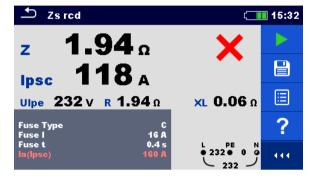
Figure 7.33: Examples of Zs rcd measurement result
