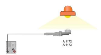
Figure 7.78: LUXmeter probe positioning
