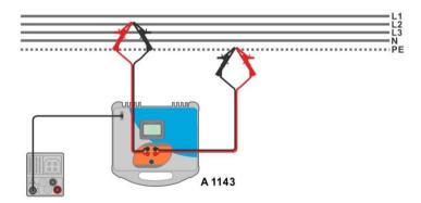
Figure 7.35: High precision Loop impedance measurement - Connection of A 1143
