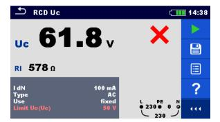
Figure 7.24: Examples of Contact voltage measurement result
