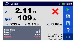
Figure 7.40: Examples of Line impedance measurement result
