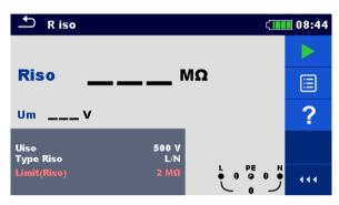
Figure 6.2: Single test start screen, example of insulation resistance measurement
