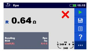
Figure 7.76: Examples of PE conductor resistance measurement result
