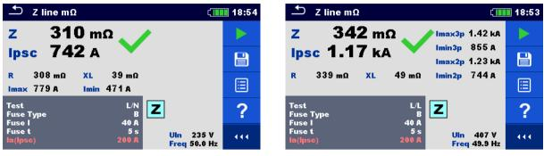
Figure 7.43: Examples of high precision Line impedance measurement result
