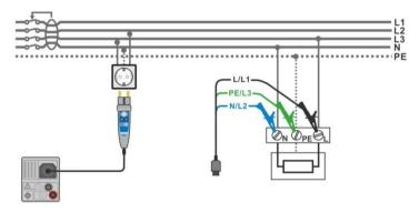
Figure 7.32: Connection of Plug commander and 3-wire test lead
