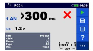
Figure 7.25: Examples of Trip-out time measurement result
