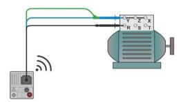
Figure 7.18: Tip commander and 3-wire test lead applications
