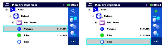
Figure 5.4: A measurement is selected in the Tree menu
