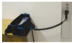
The instrument can be used even when placed in soft carrying bag – test cable connected to the instrument through the front aperture.
