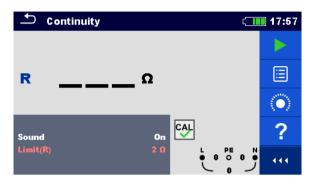
Figure 7.17: Continuity resistance measurement menu
