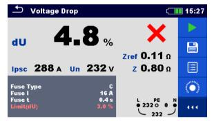
Figure 7.47: Examples of Voltage drop measurement result (STEP 2)
