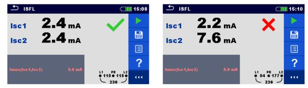
Figure 7.70: Examples of First fault leakage current measurement result
