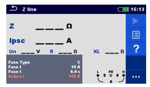
Figure 7.38: Z line measurement menu
