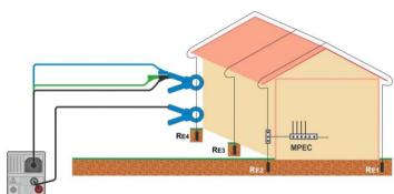
Figure 7.53: Contactless earthing resistance measurement
