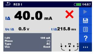
Figure 7.26: Examples of Trip-out current measurement result
