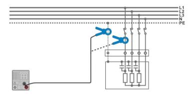
Figure 7.65: Leakage and load current measurements
