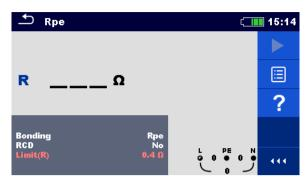
Figure 7.74: PE conductor resistance measurement menu
