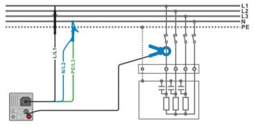
Figure 7.59: Power measurement
