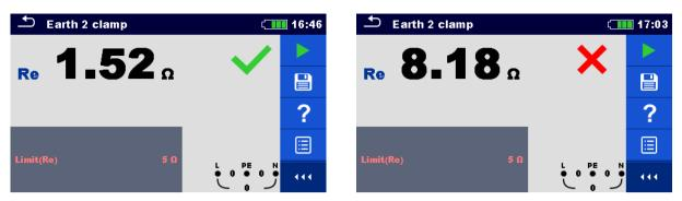
Figure 7.54: Examples of Contactless earthing resistance measurement result
