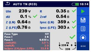
Figure 8.8: Examples of AUTO TN (RCD) measurement results
