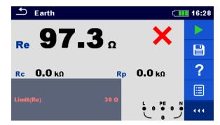
Figure 7.51: Examples of Earth resistance measurement result
