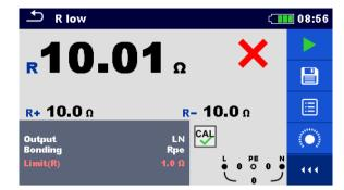
Figure 7.16: Examples of R low measurement result
