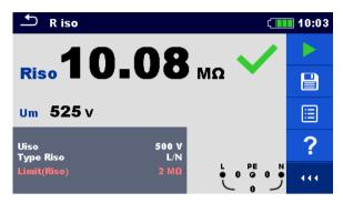
Figure 6.4: Single test results screen, example of insulation resistance measurement results
