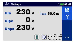
Figure 7.4: Examples of Voltage measurement in single-phase system
