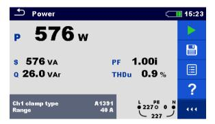
Figure 7.60: Example of Power measurement result
