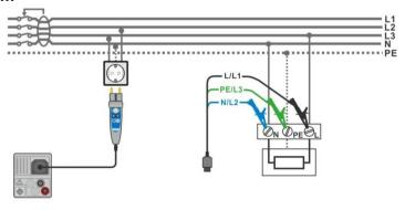
Figure 8.7: AUTO TN (RCD) measurement
