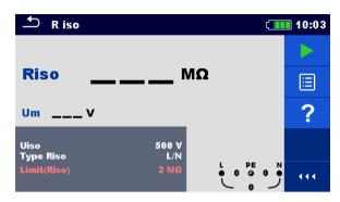
Figure 7.6: Insulation resistance measurement menu
