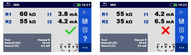
Figure 7.73: Examples of IMD test result
