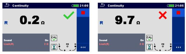
Figure 7.19: Examples of Continuity resistance measurement result
