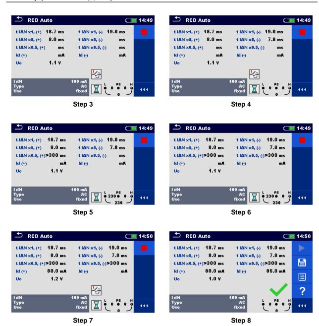
Figure 7.27: Individual steps in RCD Auto test
